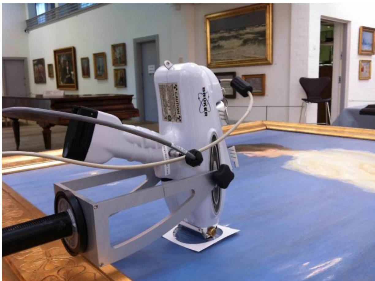
Fig. 5b. XRF analysis of a blue area in the painting P.S. Krøyer: Summer evening at Skagen . Ny Carlsberg Glyptotek, dep. at Skagens Museum. See fig. 5a.
